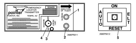
Figure 1. Pointer Model 3000-11 Emergency Locator Transmitter
