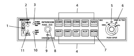
1. MARKER BEACON ANNUNCIATOR LIGHTS -- The three-light marker beacon receiver built into the KMA 26 gives a visual and aural signal when the ship's antenna passes over a 75 MHz beacon. The blue, amber, and white lights on the faceplate, as well as the audio tones, identify the beacon type.
