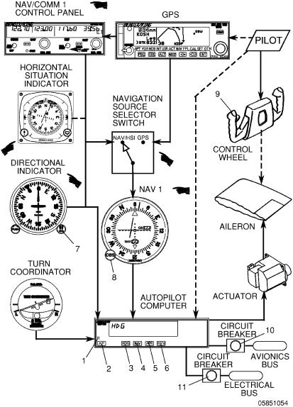
Figure 1. Bendix/King KAP 140 Autopilot, Operating Controls and Indicators (Sheet 1 of 3)
